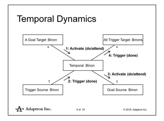
It is necessary to understand the behaviour of temporal binons to explain their role in controlling a P-A hierarchy. This a UML communication diagram to illustrate how the wave of activation travels horizontally from left to right through a hierarchical network of temporal binons. All the binons on this diagram are temporal binons.
