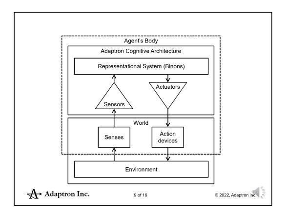
Adaptron needs to be connected to its environment via a configuration of senses and action devices.
